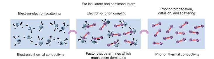
FIG. 11. Schematic role of EPC in determining which thermally conducting mechanism dominates in an insulator or semiconductor.
