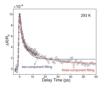
FIG. 5. Ultrafast QP relaxation processes of c-BAs at room temperature. Black circles: experimental data. The three-component (red curve) and two-component (blue curve) function fitting results.
