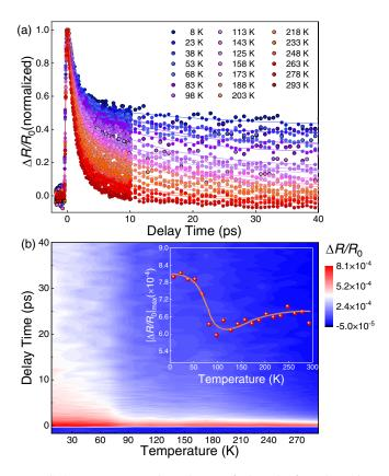
FIG. 2. Temperature dependence of the ultrafast dynamics. (a) Normalized differential reflectivity at different temperatures. Solid curves: fitting results based on Eq. (1). Note that the time step in the first 10 ps is smaller than that after 10 ps. (b) Two-dimensional color map of the QP dynamics. Inset: temperature dependence of  $|\Delta R/R_0|_{\rm max}$ . Solid curve: guide for the eyes.
