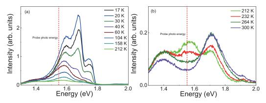
FIG. 8. Evolution of PL of *c*-BAs as a function of temperature (a) from 17 to 212 K and (b) from 212 to 300 K [44]. Red dashed line: probe photon energy of 1.55 eV. Data adapted from Ref. [44].
