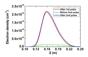
**Figure 7.** On-axis electron density of the plasma channel at different points in time: red line – after the 1st pulse, green line – before the 2nd pulse, and blue line – after the 2nd pulse.
