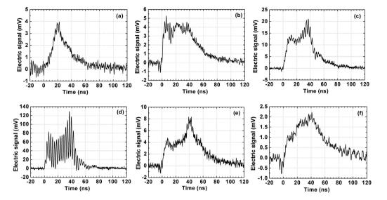
Figure 3. Electric signal of the plasma channel under f=2 m external focusing at different distances. (a) z=0 cm, (b) z=5 cm, (c) z=10 cm, (d) z=20 cm, (e) z=25 cm, and (f) z=35 cm.
