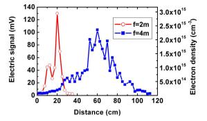
**Figure 5.** Peak electric signal (left vertical axis) and electron density (right vertical axis) of the plasma channel under initial focusing conditions f=2 m (open circle) and f=4 m (square).
