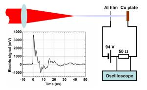
Figure 2. Setup of electric diagnostics of the plasma channel and an example of the electric signal of the plasma channel generated by a single femtosecond laser pulse.
