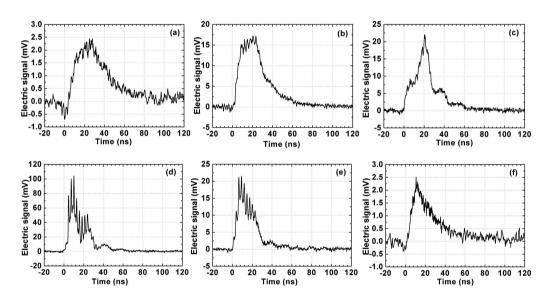
Figure 4. Electric signal of the plasma channel under f=4 m external focusing at different distances. (a) z=0 cm, (b) z=25 cm, (c) z=37.5 cm, (d) z=60 cm, (e) z=85 cm, and (f) z=112.5 cm.
