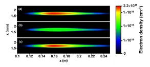
**Figure 6.** The electron density distribution of the plasma channel at different points in time: (**a**) after the first pulse; (**b**) just before the second pulse; and (**c**) after the second pulse.
