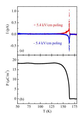
Figure 3 | Weak ferroelectricity in the Fe-MOF. (a) The pyroelectric current as a function of temperature along [012]. The sharp pyroelectric peak signals a ferroelectric transition. (b) The electric polarization along [012] obtained by integrating the pyroelectric current with time as a function of temperature. The value is an average of positive and negative poling.
