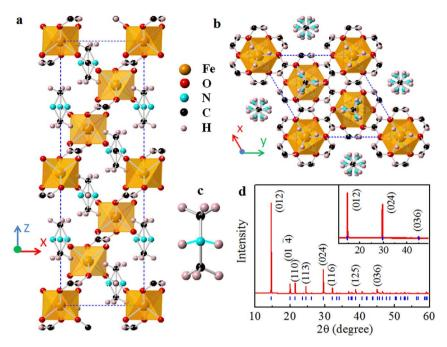
Figure 1 | Structural characterization of  $[(CH_3)_2NH_2]Fe(HCOO)_3$ . (a) Side and (b) top view of the crystalline structure. (c) The A-group cation (DMA<sup>+</sup>). (d) Powder x-ray diffraction pattern of prepared samples at room temperature. The inset shows the single crystal x-ray diffraction pattern.
