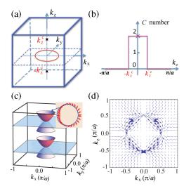
FIG. 2 (color online). Weyl nodes and gauge flux in HgCr<sub>2</sub>Se<sub>4</sub> (a) The band crossing points in the  $\vec{k}$  space; (b) The Chern number as function of  $k_z$ ; (c) The schematic plot of the band dispersion around the Weyl nodes in the  $k_z = \pm k_z^c$  plane, the inset shows the chiral spin texture; (d) The gauge flux evaluated as Berry curvature in the  $(k_x, k_z)$  plane.
