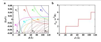
FIG. 4 (color online). Quantized anomalous Hall effect in  $HgCr_2Se_4$  thin film [30]. (a) The subband energy levels at  $\Gamma$  point as a function of film thickness. (b) The Hall conductance as a function of film thickness.
