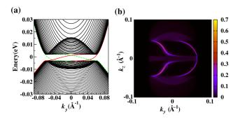
FIG. 3 (color online). Edge states and Fermi arcs of HgCr<sub>2</sub>Se<sub>4</sub> [30]. (a) The edge states for the plane with  $k_z = 0.06\pi$ . A ribbon with two edges is used, and there are two edge states for each edge (because C = 2). The states located at different edges are indicated by different line types. (b) The calculated Fermi arcs for the  $(k_y, k_z)$  side surface.
